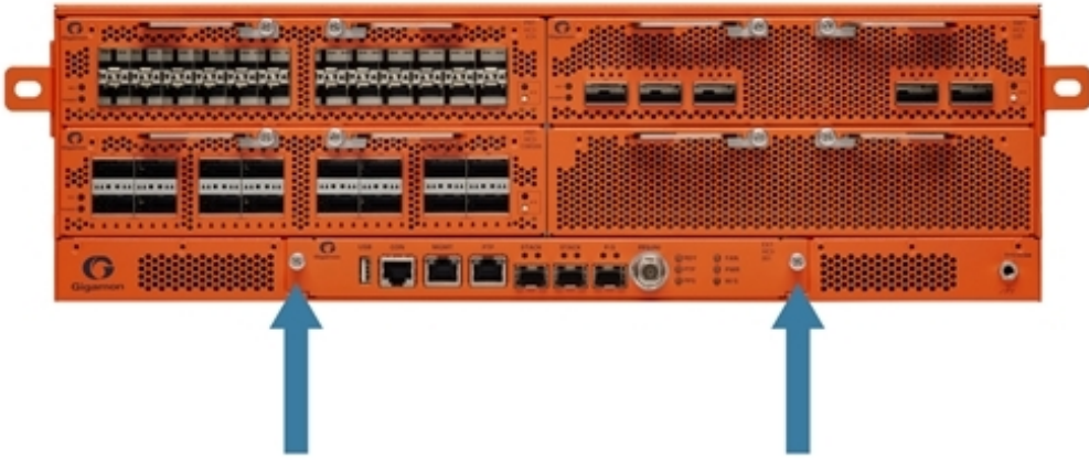
Figure 15 Extension Board Screw Location on GigaVUE-HC3 Front
