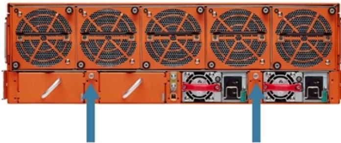
Figure 10 Fan Tray Screw Location on GigaVUE-HC3 Rear
